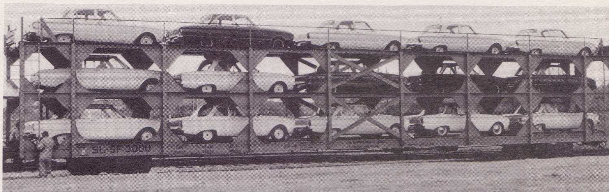
Experimental rail car designed for the movement of automobiles and capable of hauling 15 compact models or 12 ordinary-sized cars.
