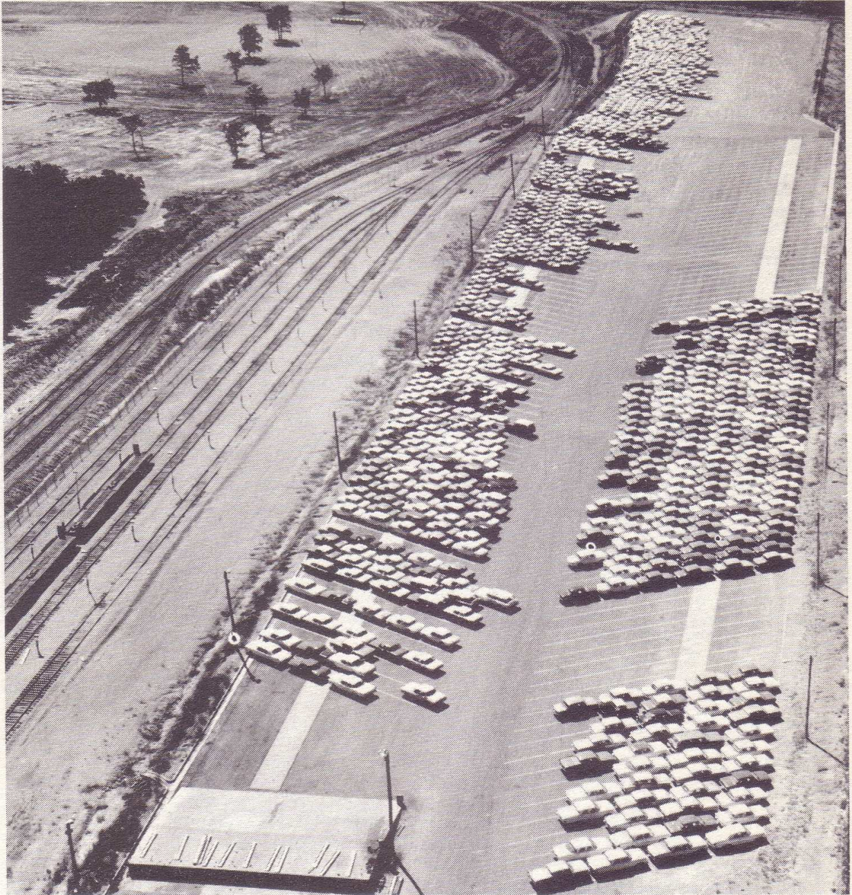
Aerial view of Company's automobile unloading facilities at Irving, Texas. Automobiles have been unloaded from multi-level railway cars which transported them from St. Louis, Mo., and await movement by highway trailers to ultimate destinations in North Texas and the Southwest.
